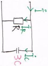
$$\cos \theta = \frac{I_R}{I} = \frac{I_R}{\sqrt{I_R^2 + I_c^2}} = \frac{V_P/R}{\sqrt{\left(\frac{V_P}{R}\right)^2 + \left(\frac{V_P}{3\omega C}\right)^2}} = \frac{V_P/R}{\sqrt{\frac{V_P^2}{R^2} + \frac{V_P^2 \cdot 9\omega^2 C^2}{9}}}$$
