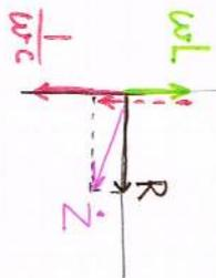
$$\begin{aligned} Z &= R + (X_L - X_C) \\ &= j\omega L + \frac{1}{j\omega C} \\ &= j(\omega L - \frac{1}{\omega C}) \end{aligned}$$
