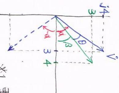
$$\dot{V} = 5 \angle 53.13^\circ \quad \dot{I} = 5 \angle 36.87^\circ$$
