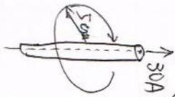
$$\text{磁界の強さ } H = \frac{I}{r} = \frac{I}{2\pi r} \quad [\text{A/m}]$$
