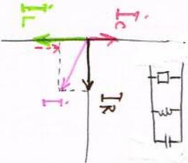
$$\frac{1}{Z} = \frac{1}{R + \frac{1}{X_L + \frac{1}{X_C}}} = \frac{1}{R + \frac{1}{j\omega L} + \frac{1}{\frac{1}{j\omega C}}} = \frac{1}{R + j\omega L + j\omega C} = \frac{1}{R + j(\omega C - \omega L)}$$
